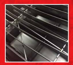
Extraction The zoned downdraft table option captures fumes and particles from beneath the cutting area.
