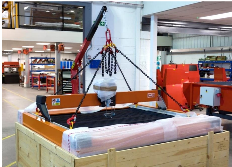
Fig 11 Lifting with the machine level
