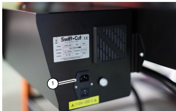
Fig 26 Control box power connection
